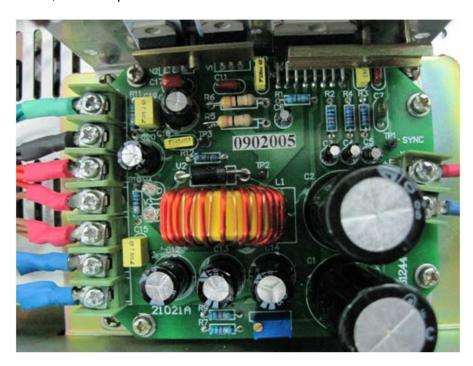
Figure 26 ±12V auxiliary power
