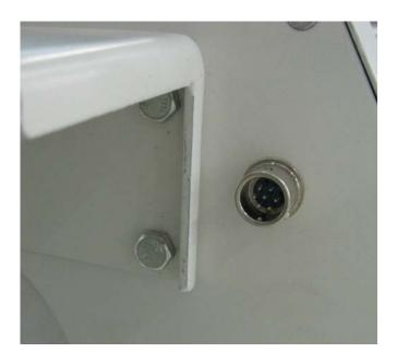
Figure 12 Data/power line interface(at the back of the operation panel)
